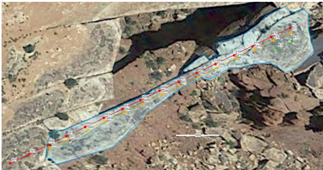
Figure 1. Musselman Arch nodal array geometry. Station names are shown with lines indicated by color: red-A, orange-B, green-C. Blue polygon outlines the arch span.
