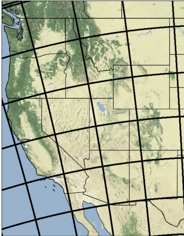
Figure 1.4: HRRR-Zarr data chunk boundaries over the western United States. Map is filled to display terrain and land cover.
